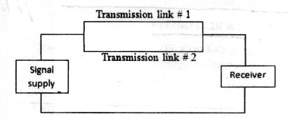
If the above circuit is left operating for a period of 1000 hours, what is the probability of it still operating at the end of this time? If transmission link # 2 is removed from service, what is the probability of the system operating at the end of a 1000 hour period? (10)
